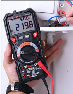
Home 220V AC voltage measurement
