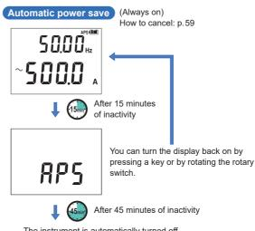
The instrument is automatically turned off. Set the rotary switch to the OFF position to restart.
