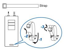
3 Attach the strap buckle to the instrument and connect it to the clip that you attached to the P2000 with the strap.
