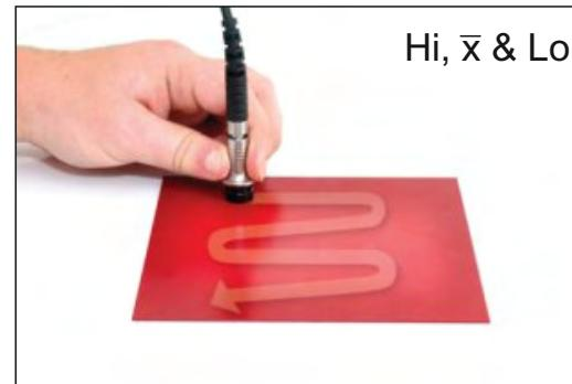
**Auto Repeat Mode:** When the probe is placed onto the coated substrate in Auto Repeat Mode, the gauge automatically takes readings at a rate of 140 per minute until the probe is removed from the substrate. Each individual reading is stored into the memory. The Auto Repeat Mode can be used to significantly speed up the inspection of large coated areas such as steel I-beams (RSJ's), tanks, ship hulls, etc.
