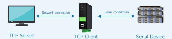
TCP Client will try establishing TCP connection with configured IP to achieve bi-directional transparent transfer between the server and serial device, and keeps retrying if failed
