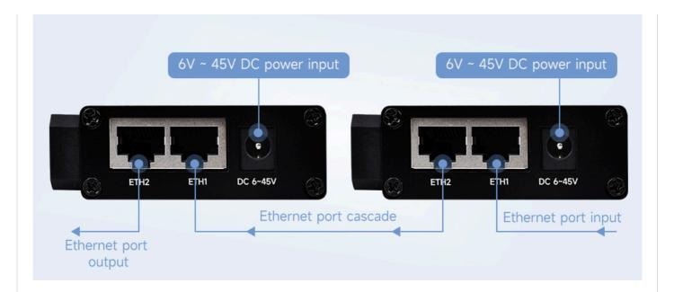
\* Note: Each module in the cascade needs to be powered individually. The working current of the module is 12V/150mA (MAX) and can be cascaded up to 8.
