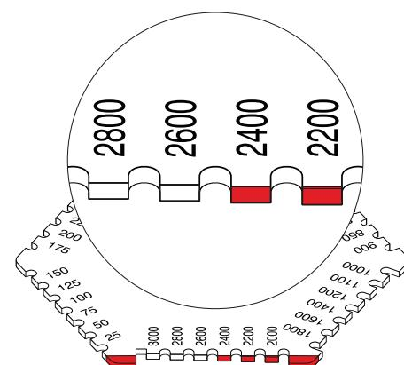
On rough surfaces, measurements will be made from the surface peaks and therefore will represent the minimum wet film thickness.
