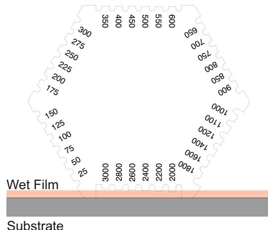
In the example shown, the wet film thickness lies between 2400µm and 2600µm.
