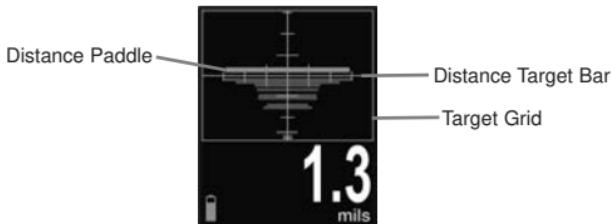
While watching the gage display, move the probe tip closer to the target, aligning the **Distance Paddle** with the **Distance Target Bar**. The optimum distance for measurement is 2 cm (3/4 inch) between the probe tip and the surface of the applied powder. Ensure the **PosiTest PC** is held perpendicular to the surface.
